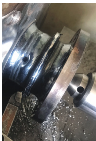
From left to right, these before-and-after photos illustrate the types of repairs done at Mile High Crankshafts. In this case, journals that had seen better days were made like-new again.
