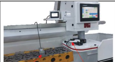
ROBINS... first Dual Axis Electronic & Bubble level (use either one) Touch off / levelling dial indicator slides on linear guideways from front to back
