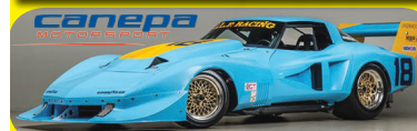
Super Vette, Riley Tube chassis, engines by Lee Muir. Ran Kinsler crossram manifold and Lucas mechanical metering.
