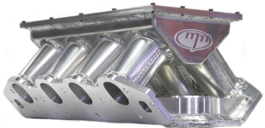
Note the precise transformation from the round throat in the plenum to the oval at the cylinder head port designed into this custom sheet-metal intake from M&M Competition Engines. CAD and computational fluid dynamics help some manifold manufacturers with their designs, but M&M relies on its years of experience to help customers make power, said Tim Linder.
